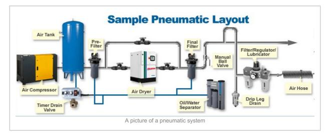
Pneumatics were one of the first original control systems. Pneumatics operate by compressing air which is then dried (to remove moisture) and sent down piping called **main lines**.
